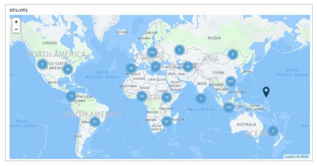
Instead of overlapping, multiple pins at the same location are displayed in a helping circle, decluttering the pins and making it easier to click or hover over them for additional information.
